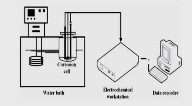
Three electrode set up
