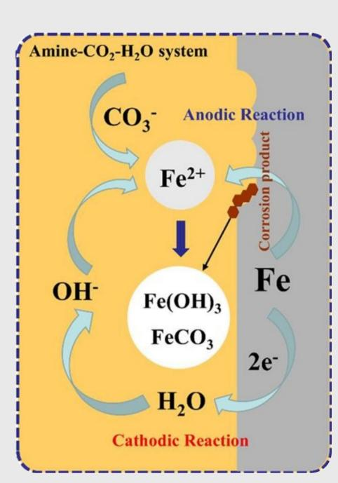
Corrosion mechanism in Amine-CO<sub>2</sub>-H<sub>2</sub>O system [2]
