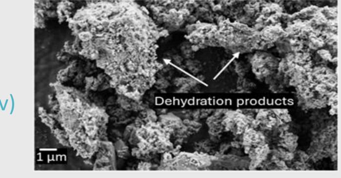
The scanning electron microscopy images reveals that C-S-H phases in (v) unexposed Portland cement powder and, (vi) CO<sub>2</sub> exposed steel infused cement dehydrated under high temperatures, forming a flocculent structure.
