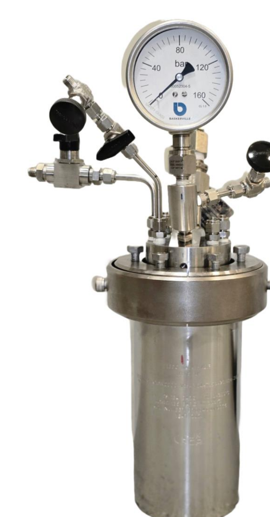
Autoclave for tests in simulated well conditions
